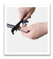
**STEP 4:** Test with Press Gauge.
